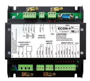
ECON-4 is digital speed governor dedicated for speed control of gas or diesel engines. ECON-4 guarantees precise and fast speed control in island and network parallel operation. ECON-4 can control different types of actuators which makes it a general speed controller for almost every actuator on the market for engines in range of multiple MWel.
